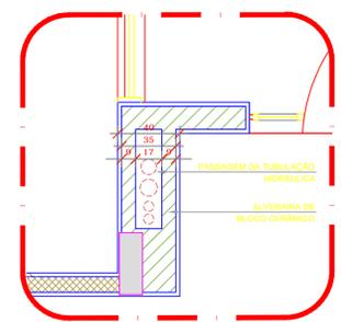
**2 DETALHE - SHAFT HIDRÁULICA**
